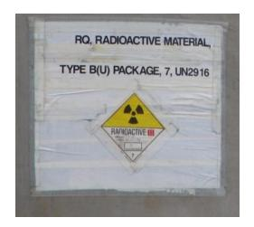
What is wrong here? Is anything else required when a label is placed on a non-contrasting background? Looking at 49 CFR 172.406(d), we find that a dotted
